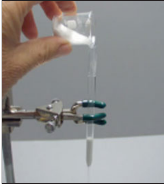
This photo is of a very small chromatography column being filled with silica gel. Many separatory columns are much larger, but the same material is used to pack the columns.
