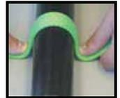
**Rope Lanyard** – Rotate the rope lanyard while inspecting from end-to-end for any fuzzy, worn, broken or cut fibers. Weakened areas from extreme loads will appear as a noticeable change in original diameter. The rope diameter should be uniform throughout, following a short break-in period.
