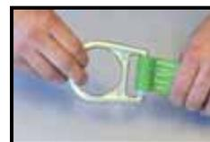
**Attachment of Buckles** – Inspect for any unusual wear, frayed or cut fibers, or broken stitching of the buckle or D-ring attachments.
