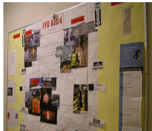
An Acceptable bulletin board. Materials are secured on all corners and there is no excess accumulation or layering of posted materials.
