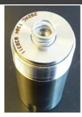
Place the bottom pressure plate on top of the rupture disc, so that the part number is facing up. Set the spring in the depression.
