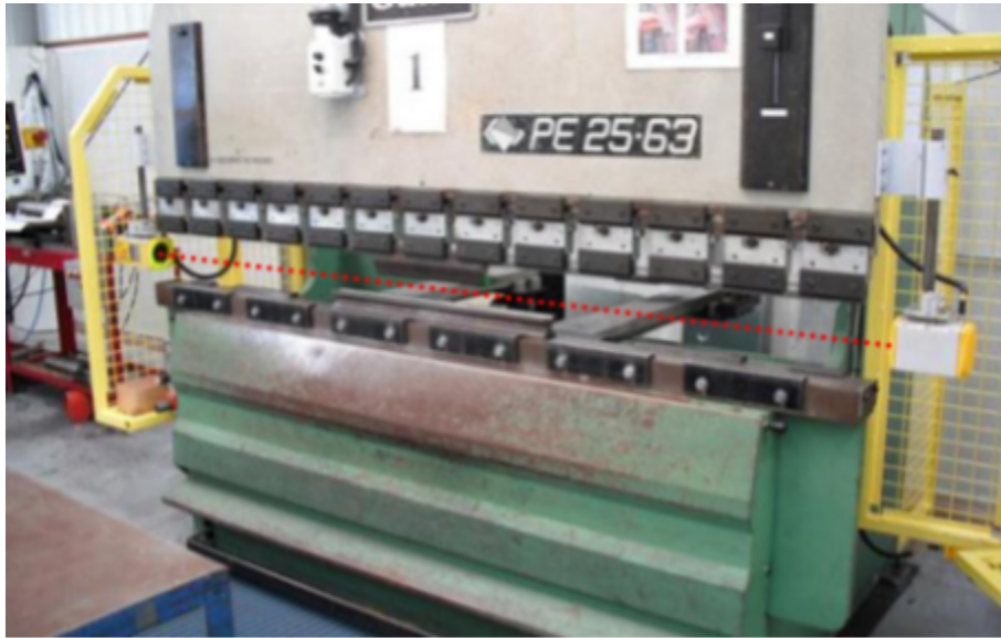
Optical light beam on a press.
