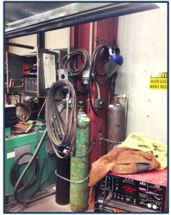
Welding-gas cylinders must be separated by a distance of 20 feet, or by a noncombustible partition 60 inches high or taller.
