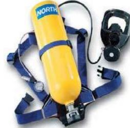
**Supplied-Air Respirator** - A hose-mask respirator equipped with a face piece, breathing tube, safety harness, and safety line. The respirable air is supplied through an air hose connected to a compressed-air cylinder or air compressor. Generally, this type of respirator is not issued to Berkeley personnel.
