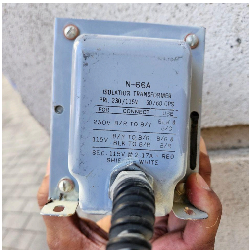
Left: Photo of N-66A Isolation Transformer before the incident.
