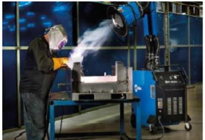
Welding fumes being pulled out by a snorkel exhaust
