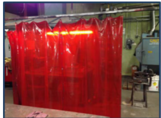
Welding area, with the welding curtain separating work area from the rest of the space
