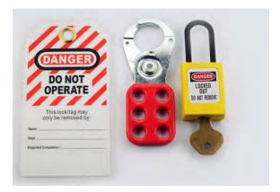
indicate different shifts, types of crafts, or lock owners. When more than one worker is servicing a piece of equipment that must be locked out, a lockout adapter hasp is used which allows all the workers to place their locks on the disconnecting means. Each worker puts one of their locks on every isolation device prior to starting work on a machine. After the work is completed, each worker removes their lock(s) and the machine is then returned to service.
