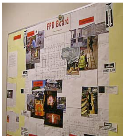
An acceptable bulletin board – Materials are secured on all corners and there is no excess accumulation of posted materials.
